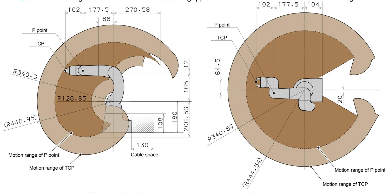
Outline drawing of COBOTTA with an electric gripper for COBOTTA and an AF camera mounted
