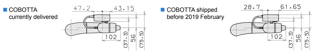
Dimensions of screw holes for fixing COBOTTA (common in products with or without option)
