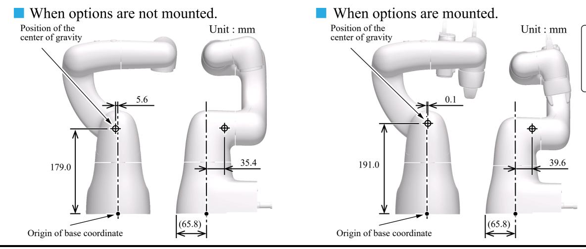
Position of the center of gravity (COBOTTA packing posture with packing material used for shipments up to Feb 2019)
