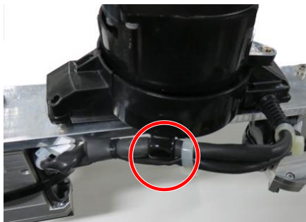
Example of fixing the D1 connection cable.
