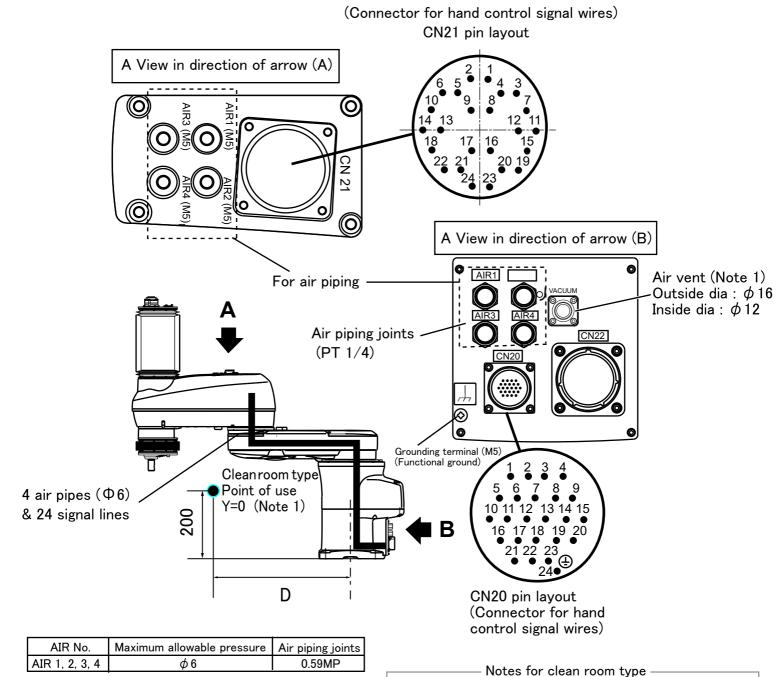
(Note 1) Dimension D at point of use for clean room type (distance from the rotation center of the first axis) D = 500 mm
