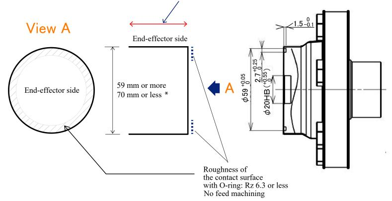
\* If the cabling length is 70 mm or more, secure a wider cabling space to the end-effector side so that the wiring and piping are not suddenly bent. (Refer to the figure below.)
