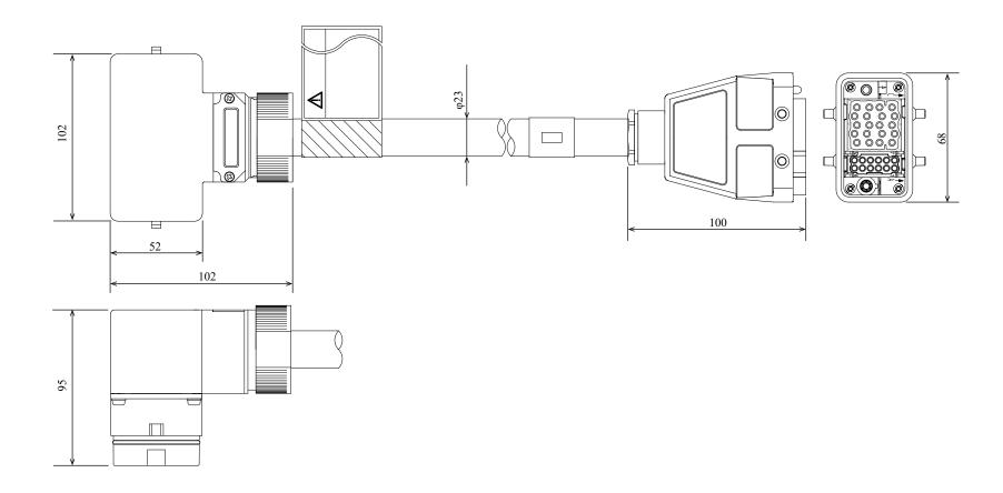
The bending radius (internal) of a motor & encoder cable should be at least 33.8 mm when the cable is stationary, and at least 225 mm when it is movable. Excessively bending will result in broken lead wires.
