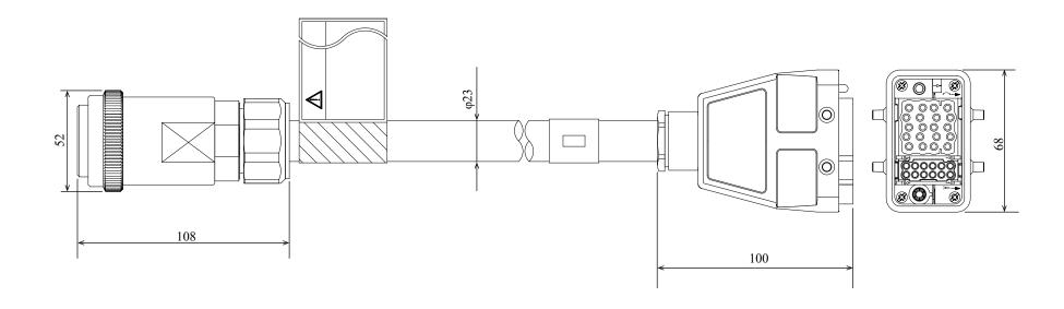
The bending radius (internal) of a motor & encoder cable should be at least 33.8 mm when the cable is stationary, and at least 225 mm when it is movable. Excessively bending will result in broken lead wires.
