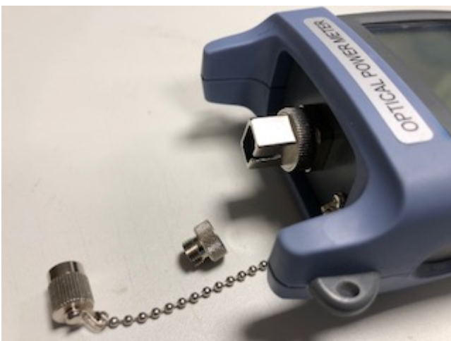
Fig. 48: OPM with SC adapter screwed on
