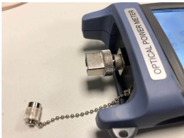
Fig. 49: OPM with FC and SC adapter screwed on - WRONG
