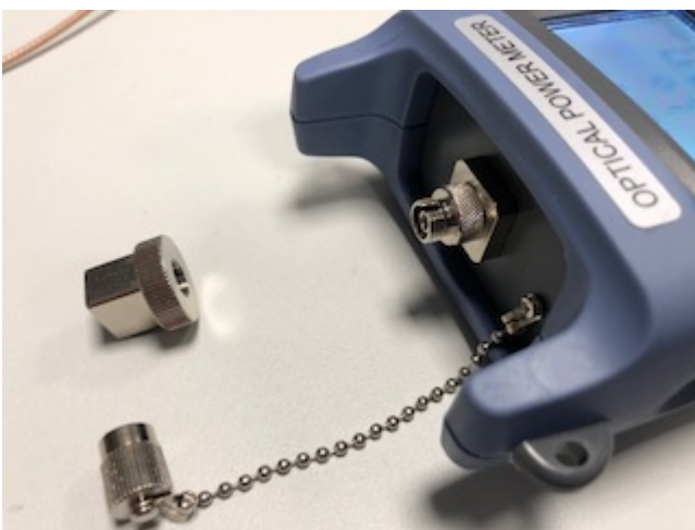
Fig. 47: OPM with FC adapter screwed on
