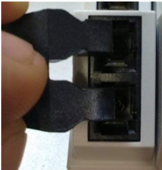
Figure: Blind plugs in unused sockets
