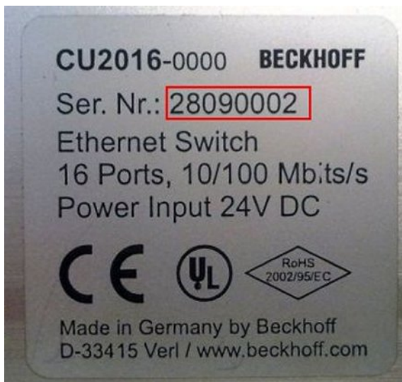
Fig. 3: CU2016 switch with serial/ batch number
