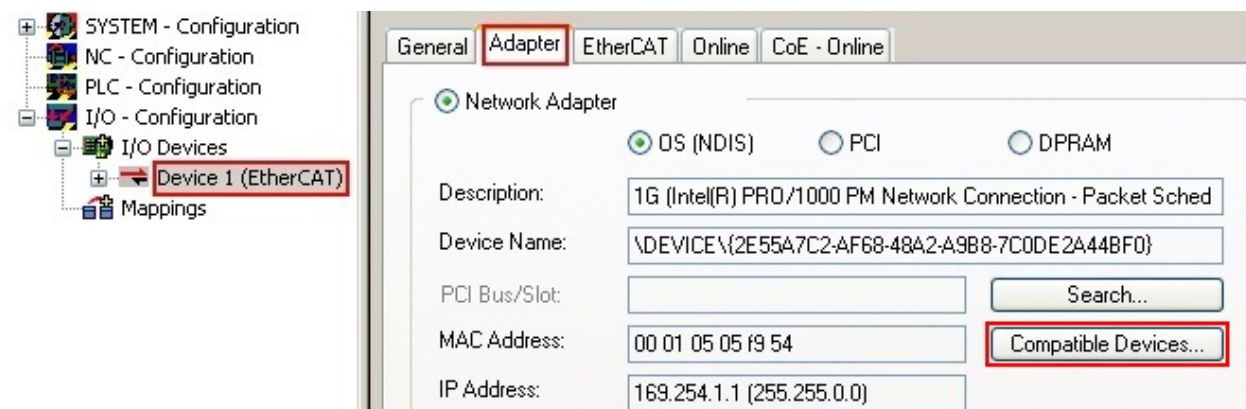
Fig. 64: EtherCAT device properties(TwinCAT 2): click on „Compatible Devices...” of tab “Adapter”
