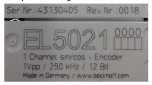
Fig. 41: EL5021 EL terminal, standard IP20 IO device with serial/ batch number and revision ID (since 2014/01)
