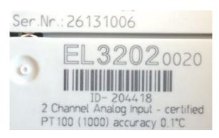
Fig. 44: EL3202-0020 with serial/ batch number 26131006 and unique ID-number 204418
