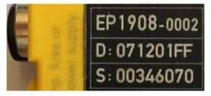
Fig. 46: EP1908-0002 IP67 EtherCAT Safety Box with batch number/ date code 071201FF and unique serial number 00346070
