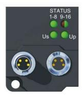
Fig. 7: EP2316-0008 - Status LEDs
