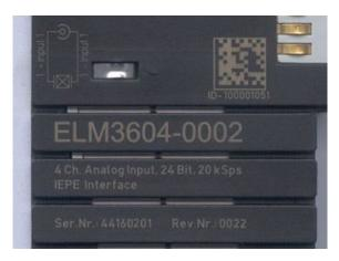
Fig. 48: ELM3604-0002 terminal with unique ID number (QR code) 100001051 and serial/ batch number 44160201
