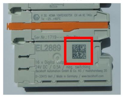
Fig. 49: BIC as data matrix code (DMC, code scheme ECC200)
