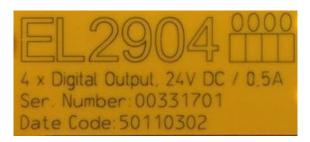
Fig. 47: EL2904 IP20 safety terminal with batch number/ date code 50110302 and unique serial number 00331701
