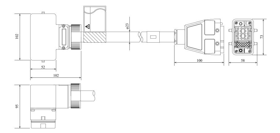
The bending radius (internal) of a motor & encoder cable should be at least 33.8 mm when the cable is stationary, and at least 225 mm when it is movable. Excessively bending will result in broken lead wires.
