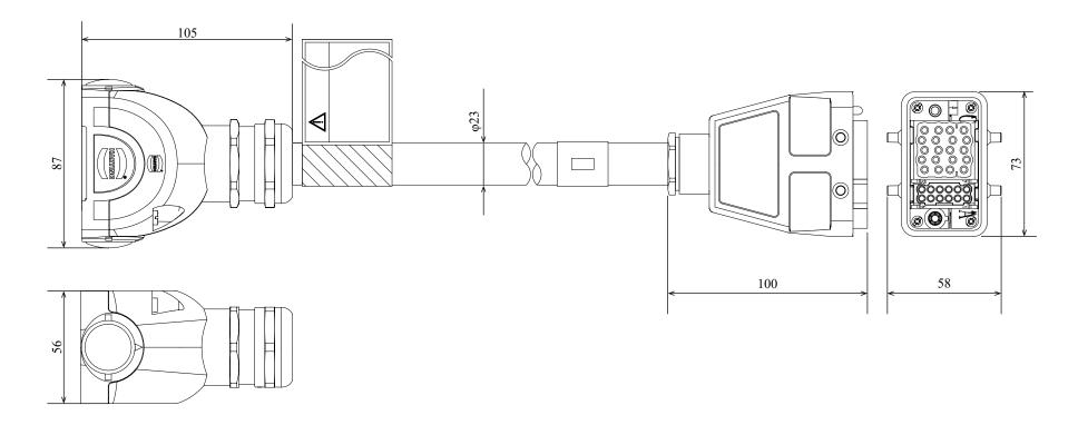
The bending radius (internal) of a motor & encoder cable should be at least 33.8 mm when the cable is stationary, and at least 225 mm when it is movable. Excessively bending will result in broken lead wires.
