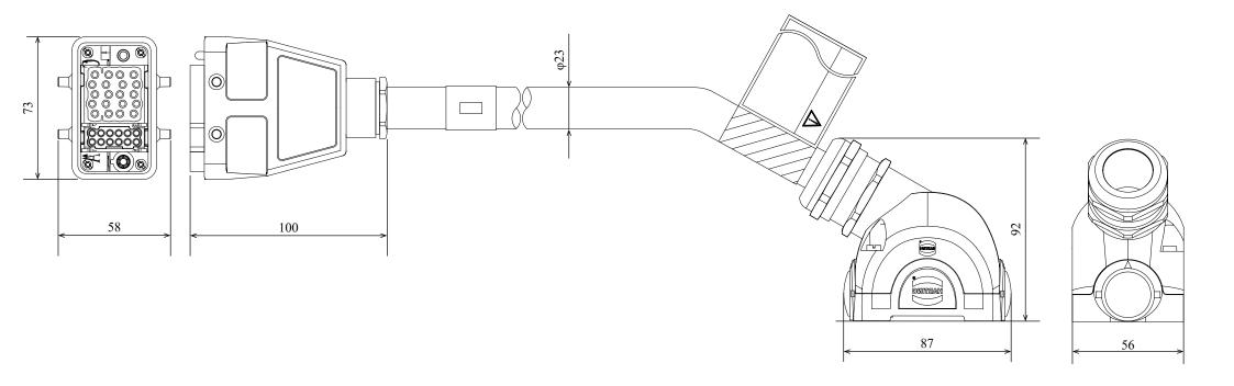
The bending radius (internal) of a motor & encoder cable should be at least 33.8 mm when the cable is stationary, and at least 225 mm when it is movable. Excessively bending will result in broken lead wires.
