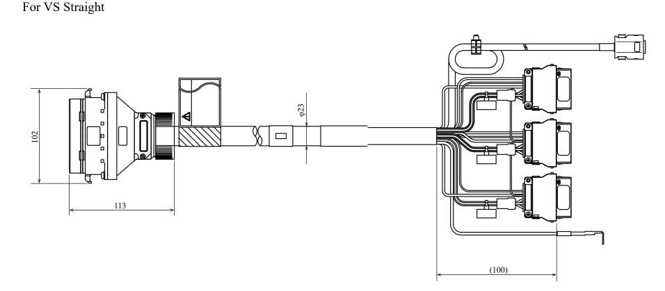
The bending radius (internal) of a motor & encoder cable should be at least 33.8 mm when the cable is stationary, and at least 225 mm when it is movable. Excessively bending will result in broken lead wires.
