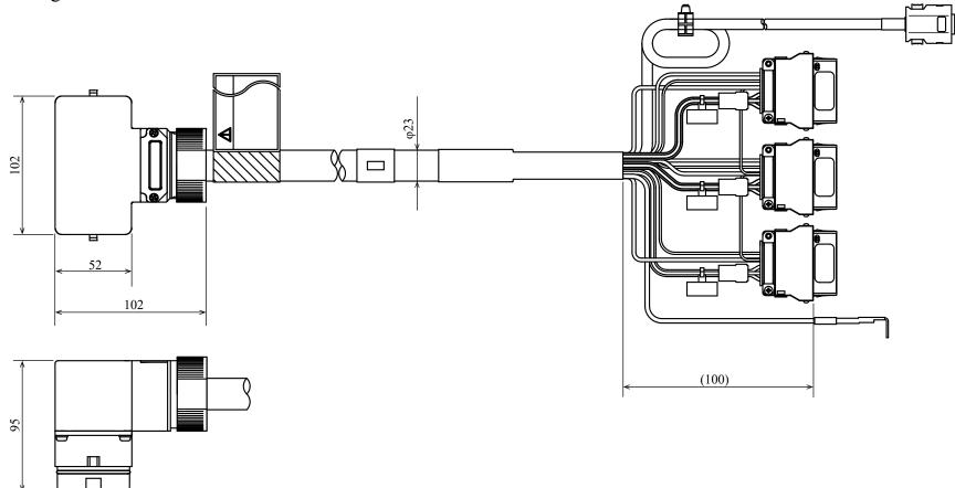
The bending radius (internal) of a motor & encoder cable should be at least 33.8 mm when the cable is stationary, and at least 225 mm when it is movable. Excessively bending will result in broken lead wires.
