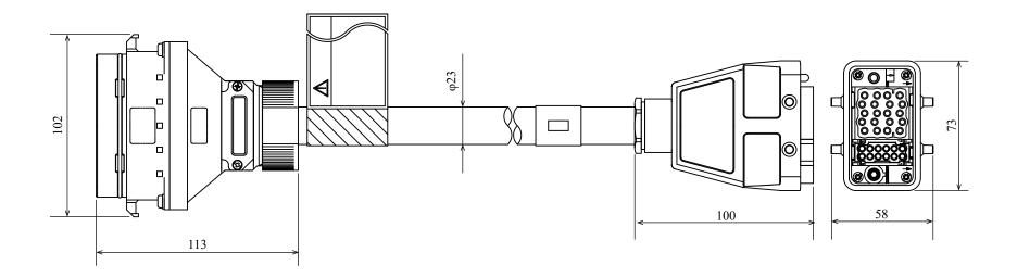
The bending radius (internal) of a motor & encoder cable should be at least 33.8 mm when the cable is stationary, and at least 225 mm when it is movable. Excessively bending will result in broken lead wires.
