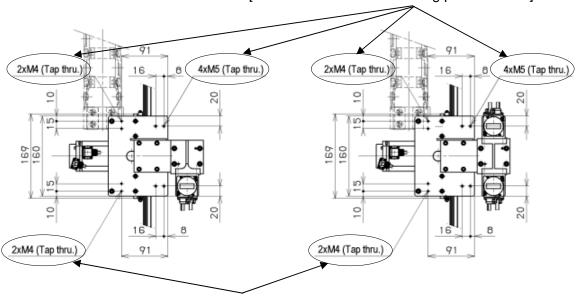
When using this screw hole, fix with a screw length of [the thickness of the mounting part + 10 mm] or
