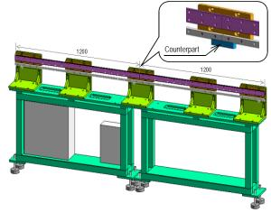
• When the rack gears are engaged, the gap between the rails should be 1mm or less.
