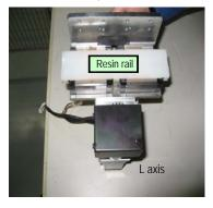
Insert the L axis to the rail with the resin rail attached so that the slider ball of the L axis does not come out.
