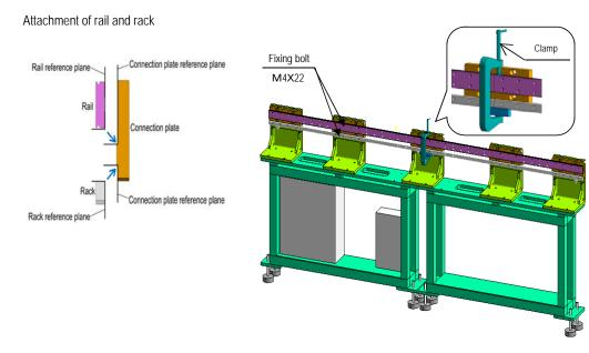
• Adjust the reference planes of the rail and rack to the reference plane of the connection plate and fix them. At that time, make the reference plane of the connection plate contact the reference planes of the rail and rack with small clamps with a clamp force of 2300N or moreso that no difference of level is found in the joint of the rails. When clamping, take measures to avoid damage to the rails.
