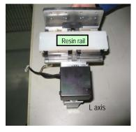
Insert the L axis to the rail with the resin rail attached so that the slider ball of the L axis does not come out.
