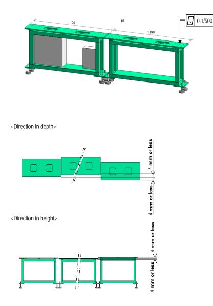
Fix the supports of the first frame temporarily.
