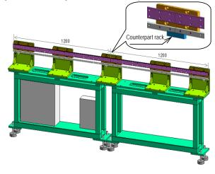
• When the rack gears are engaged, the gap between the rails should be 1mm or less.
