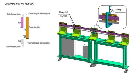
• Adjust the reference planes of the rail and rack to the reference plane of the connection plate and fix them. At that time, make the reference plane of the connection plate contact the reference planes of the rail and rack with small clamps with a clamp force of 2300N or moreso that no difference of level is found in the joint of the rails. When clamping, take measures to avoid damage to the rails.
