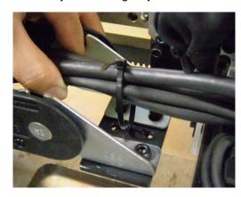
Wrap the L-axis motor cable together with the connector part of the encoder cable with a sheet, and then fix them into the cableveyor mounting stay cable ties.
