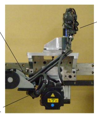
Wrap the Z-axis motor cable together with the connector part of the encoder cable with a sheet, and then fix them into the side of the Z-axis motor with cable ties.
