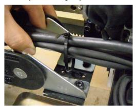
Wrap the L-axis motor cable together with the connector part of the encoder cable with a sheet, and then fix them into the cableveyor mounting stay cable ties.
