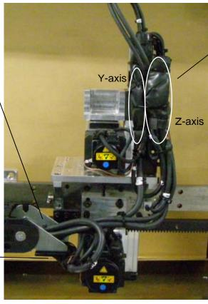
For the Y-axis and Z-axis, wrap each motor cable together with respective encoder cable's connector part with a sheet, and then fix them into the cable fixing stay with cable ties.
