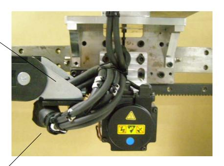
For the L-axis and S-axis, wrap each motor cable together with respective encoder cable's connector part with a sheet, and then fix them into the cableveyor mounting stay with cable ties.
