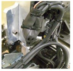
Fix the motor and encoder cable into the cableveyor mounting stay with a cable tie.
