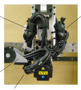
Wrap the L-axis motor cable together with the connector part of the encoder cable with a sheet, and then fix them into the cableveyor mounting stay cable ties.
