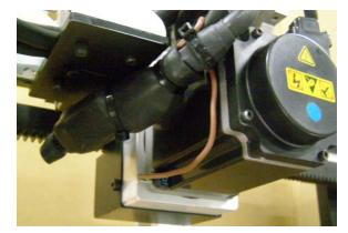
Wrap the S-axis motor cable together with the connector part of the encoder cable with a sheet, and then fix them into the side of the Z-axis bracket with cable ties.
