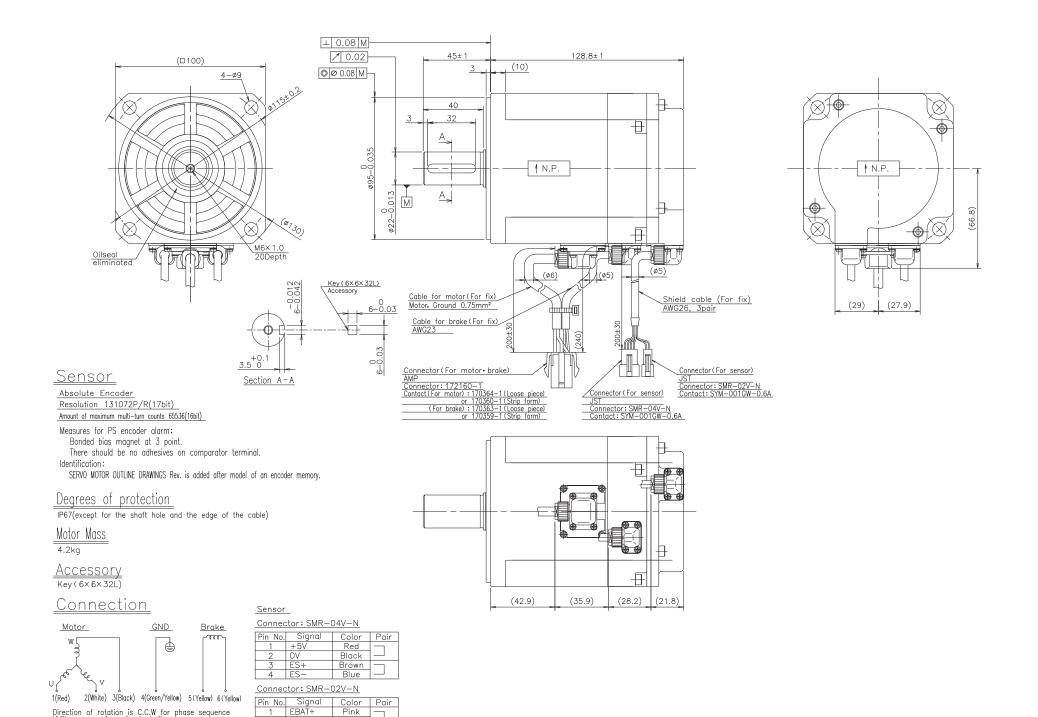
Direction of rotation is C.C.W for phase sequence UVW, as seen from front shaft.
